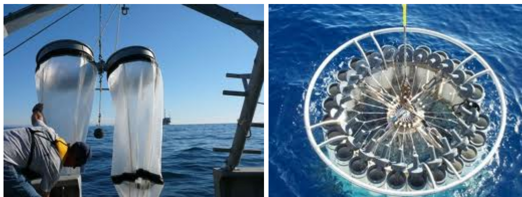
(a) Plankton tow net, 153-m pore size, 0.5-m diameter (D:L=1:3) (b) Multiple opening/closing net system
